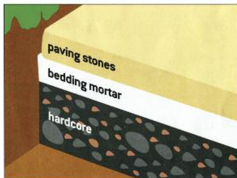
▲ (fig. 3) Compacted hardcore flattened with a powered wacker plate forms the solid, flat sub-base necessary for the bedding mortar and paving. NOTE: the layers on this diagram are not to scale.
