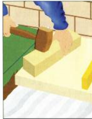
▲ (fig. 5) The slab can be gently tapped until they are the correct level.
