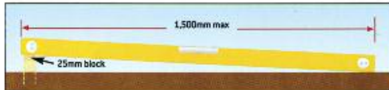
▲ (fig. 1) You must allow for a slope on the patio to make sure water drains away from your house. Allow a 25mm drop for every 1,500mm of patio.
