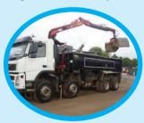
Passengers on Mobile Machinery Self-propelled work equipment is often incorrectly used to carry passengers. A recent incident provides an example of this, where two workers were observed riding on a forward tipping site dump truck, designed for one driver and no passengers.
