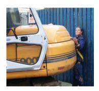
Never except a lift or give a lift to someone on an item of plant unless a proper passenger seat has been fitted by the machine manufacture for this purpose.
