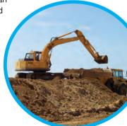
as is safe/practicable and keeping the load low to the ground. When placing the load into position, engine revs should be lowered to tortoise mode and the machine's boom and dipper manipulated to move the load into position. At all times, the load must remain freely suspended.
