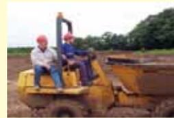
Never accept a lift on an item of plant unless a proper passenger seat has been fitted by the machine manufacturer for this purpose.
