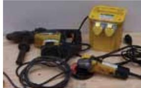
Ensure all plugs and leads are in good condition and free from defect.
