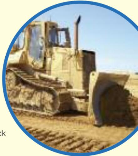
When travelling, the dozer blade should be kept at its lowest possible position to allow maximum operator vision, and machine stability. If a tractor dozer is employed on clearing scrub or felling trees it should be provided with adequate driver protection Falling Object Protection Structure (FOPS) cab.
