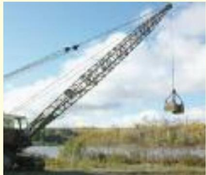
Dangerous overhangs must not be created on a high work surface, the wheel, or tracks of the machine should be positioned at 90° to the workface to enable quick withdrawal if necessary. In excavating the type of soil should be taken into account in determining a safe position for the machine.
