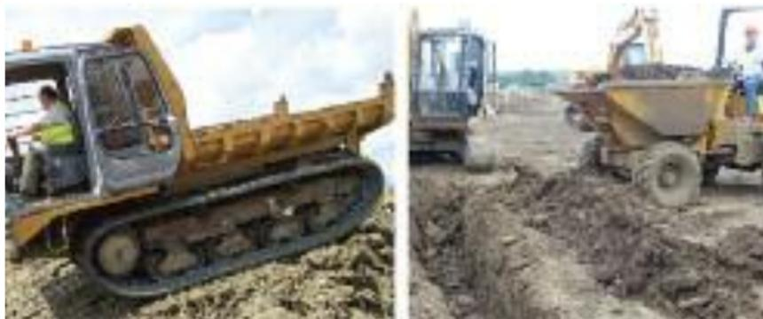
The site dumper should be operated within its capabilities with regards to handling and braking. This will include: regulating the speed to suit the ground conditions and load being carried; maintaining safe braking distances and never braking suddenly in wet, icy or muddy conditions. Never exceed the maximum stated gradients specified by the OEM; and avoiding turning across gradients.
